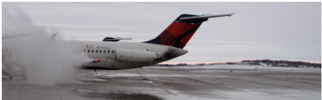
An aircraft being deiced in the winter at DCRA. DCRA has an extensive glycol management system to ensure affluent does not adversely impact local water resources.
